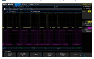
SDS1000X/SDS1000X+ displays the decoding through the events list. Bus protocol information can be quickly and intuitively displayed in table form.
