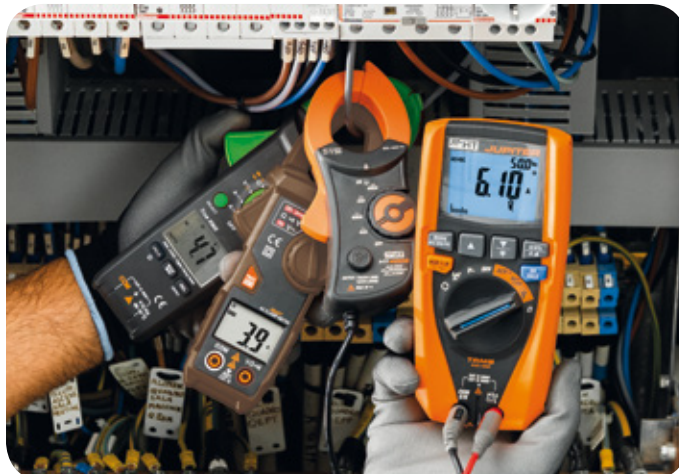
Measurement comparison: 3.9A: with RMS clamp - 4.7A: with TRMS clamp 6.1A: correct reading with AC+DC TRMS clamp.
