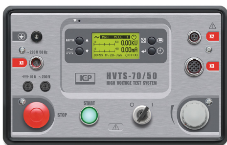
HVTS-70/50 control panel
